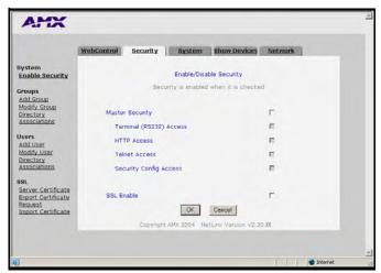
FIG. 48 Security tab - showing NetLinx Master security options
